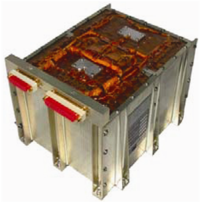
Figure 6. 36 Ah lithium-ion battery.
